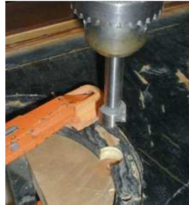
Fig. 4.2. Drilling relief holes for back-wired drivers in early cabinets.
