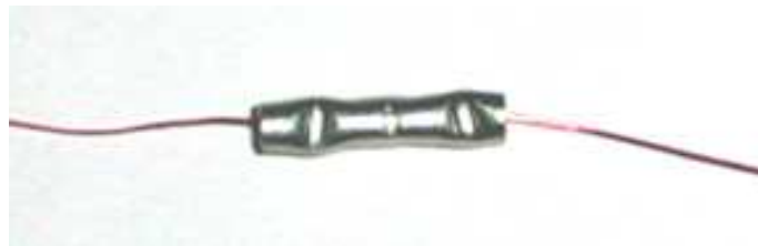
Fig. 4.3. Joining 0.0045-in.diameter wires with a crimp connector.
