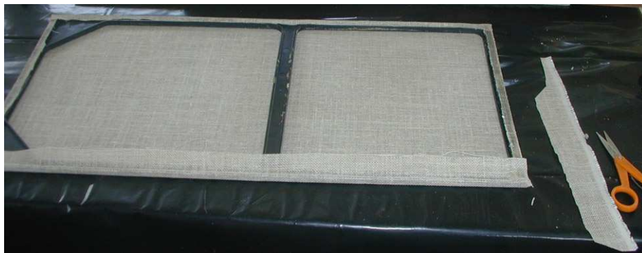
Fig. 3.20. Attaching grille cloth with gel contact cement.
