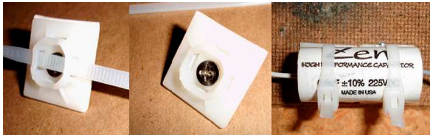
Fig. 3.18. Convenient coil and capacitor mounting bracket.
