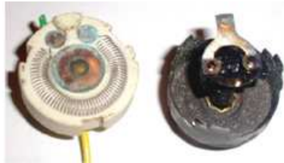
Fig. 3.12 Illustration of mild corrosion
