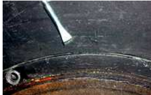
Fig. 3.2. Using a paint can opener to lift the woofer from its back bore.
