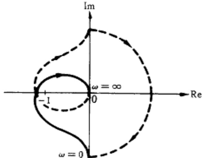
(b)  $G(s) = \frac{K}{s(1+T_1s)(1+T_2s)} ; T_1, T_2 > 0$
