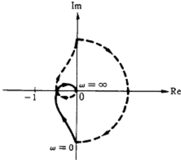
(a)  $G(s) = \frac{K}{s(1+T_1s)(1+T_2s)} ; T_1, T_2 > 0$
