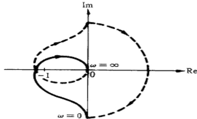
(b)  $G(s) = \frac{K}{s(1+T_1s)(1+T_2s)} ; T_1, T_2 > 0$
