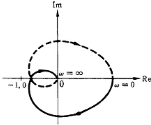
(c)  $G(s) = \frac{K}{(1+T_1s)(1+T_2s)(1+T_3s)}$  ;
