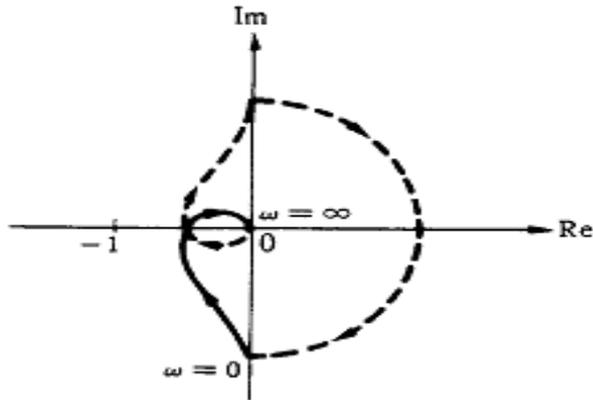
(a)  $G(s) = \frac{K}{s(1+T_1s)(1+T_2s)} ; T_1, T_2 > 0$
